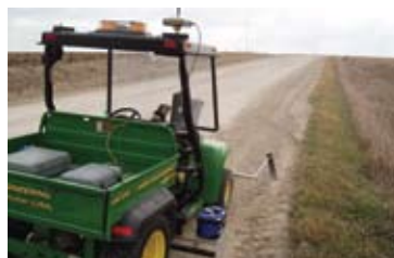
ATV with GPS and laser profiler
