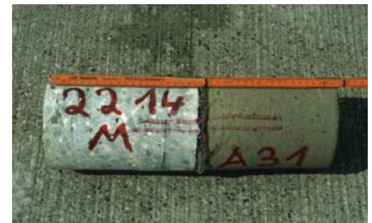
Figure 1. Core from Germany showing nonwoven geotextile interlayer between surface concrete (left) and cement-treated base (right)
